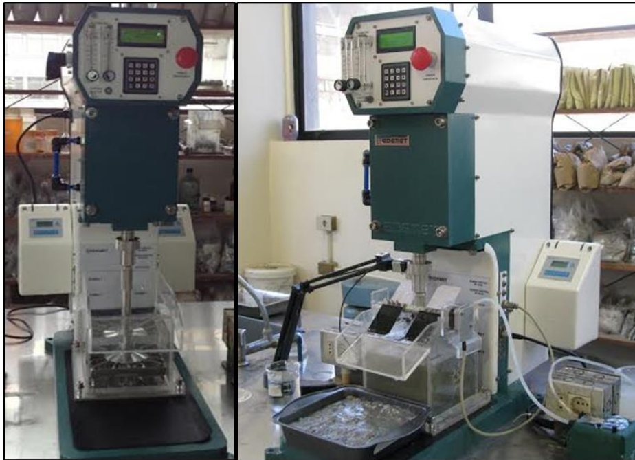
Figure 1 Flotation unit shown idle (left) and in 3-phase operation (right)
