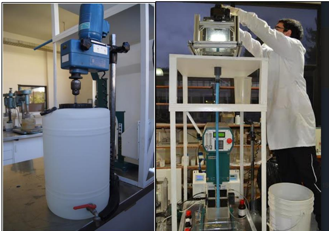
Figure 2 Arrangements used for preparation and storage of frother solutions (left), and for installation of apparatus for measuring bubble size (right)
